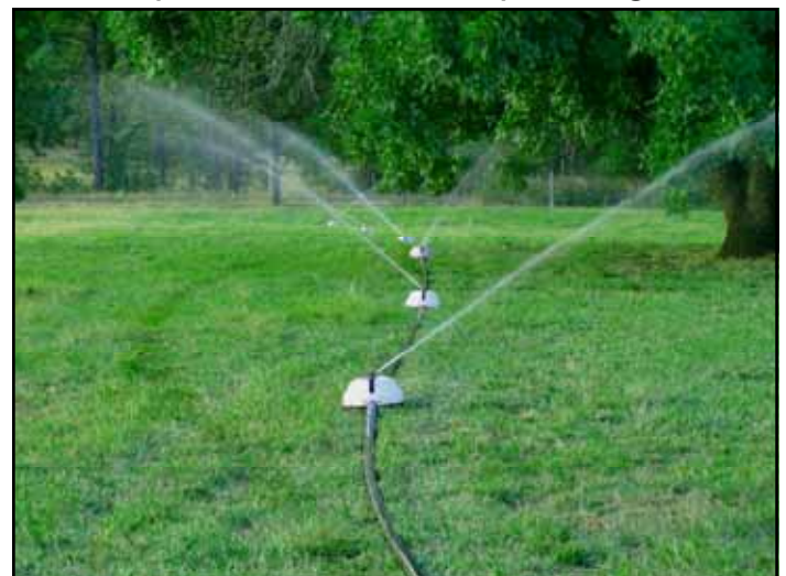
Irripod installed and operating:
