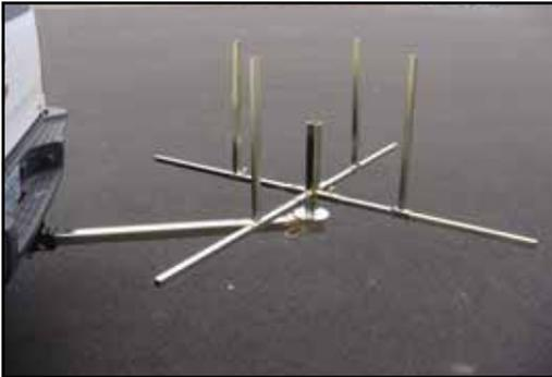
Step 4: Adjust the vertical spokes position and put on your coil of tubing. Tighten down the thumb screws.
