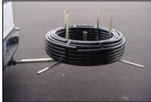
Step 5: Install four horizontal spokes onto the vertical spokes. These keep the tubing from flipping up while dispensing.
