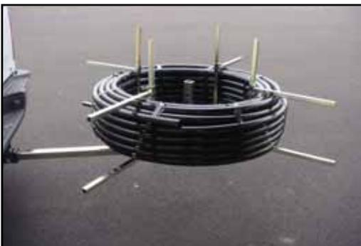
Step 6: Cut the tape on the tubing and dispense. Two methods can be used:
