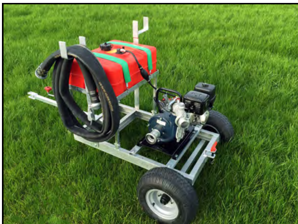
Booster Pump Cart with Honda GX gas engine:
