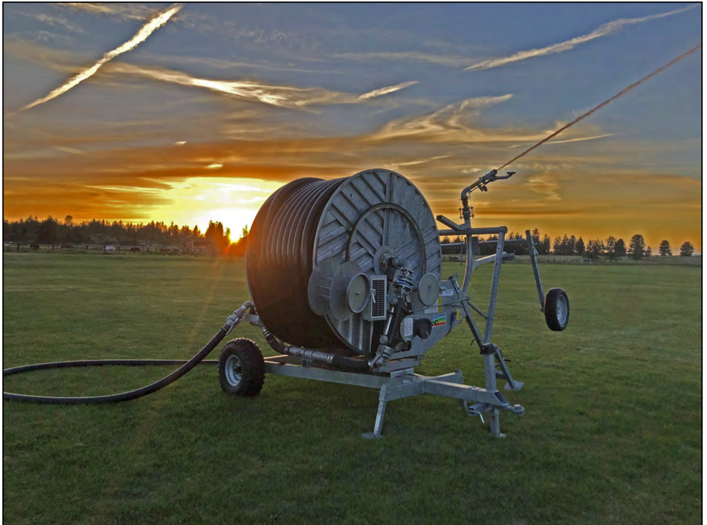
Silver series with booster pump and shut off kit near the end of run on a polo field.
