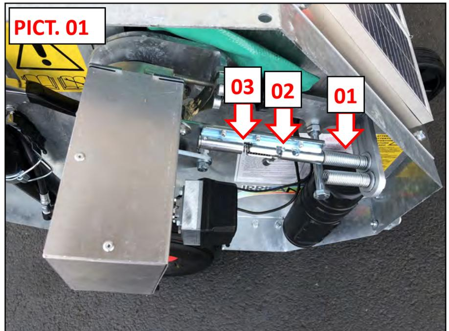
When the latch in pict. 01 is in position 02 and is inserted into the inner spring (01), the electric motor is engaged. This is the right position when irrigating and in transport position.
