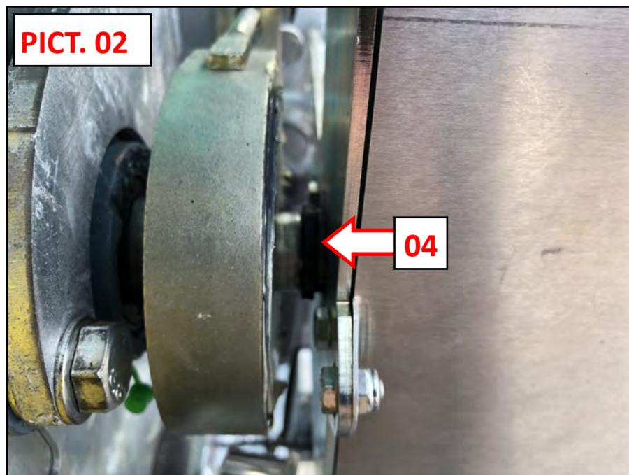
When the motor is engaged, the bracket flange on which it's mounted is very close to the brake drum, and the motor is on the square part of the drive shaft: pict. 02 position 04.
