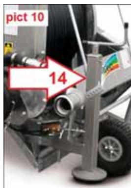
13. Anchoring "L" profile 14. Rear lifting jack 15. Diaphragm valve 16. Pressure gauge
