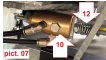
10. Brass (switch) valve 11. Irrigation position (toward the sprinkler cart) 12. Stop position (toward the drawing bar)
