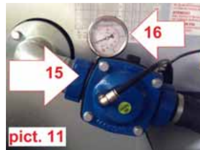
13. Anchoring "L" profile 14. Rear lifting jack 15. Diaphragm valve 16. Pressure gauge
