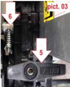
5. Engage/disengage lever: working and transport position
