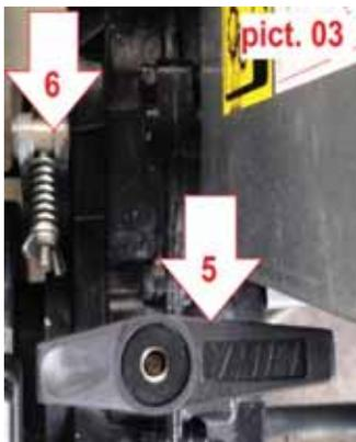
In case you can't engage/disengage the gear box moving the lever directly you can turn a bit the drum by using the hand wheel on the pto shaft: look at " 3.1 MACHINE SET UP ON THE FIELD, point 4.
