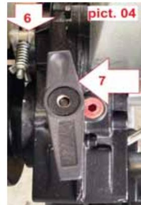
7. Engage/disengage lever: pulling out position
