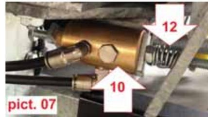
10. Brass (switch) valve      11. Irrigation position (toward the sprinkler cart)
