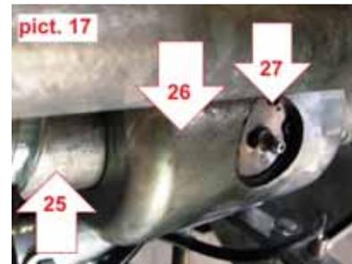
**It's necessary to lubricate every 50 working hours**
