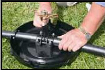
Screw sprinkler into sprinkler riser.
