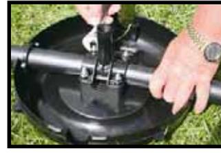
Select the saddle to fit your sprinkler, install rubber O-ring on saddle, locate saddle onto pipe and cross tee anchor – ensure fastening nuts are tightened evenly.
